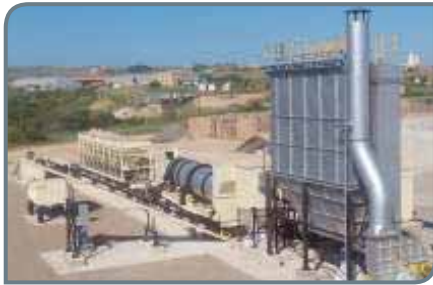
ASPHALT DRUM MIX PLANT
