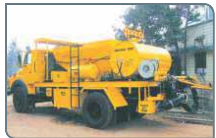
POTHOLE REPAIRING MACHINE
